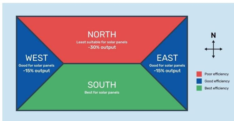
*The graphic shows ballpark figures for the output losses experienced by pointing your panels in a direction other than south. Source: Solar Reviews*
